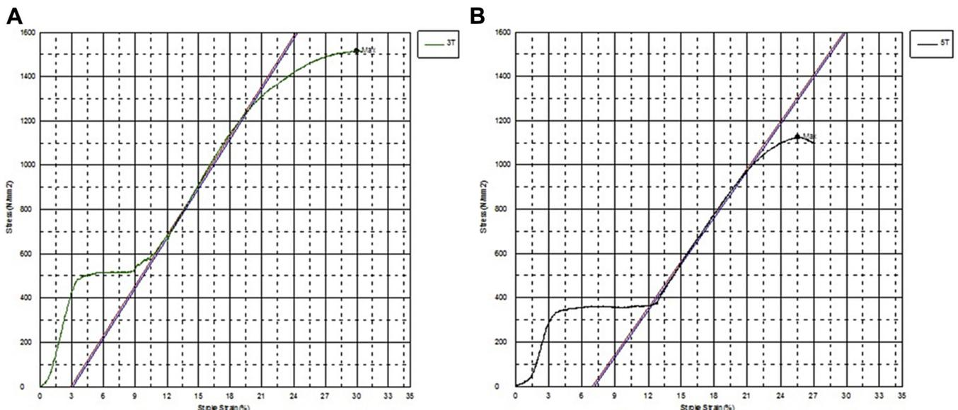
**Fig. 1.** Stress/strain curves in tensile test at T0. (A) Thermoelastic NiTi wire. (B) Pseudoelastic NiTi wire. The red line in the figures determines the slopes of the plots for continued loading beyond the pseudoelastic region.
