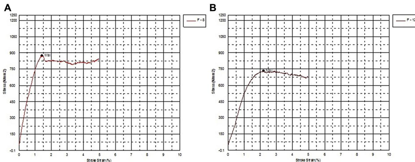
**Fig. 4.** Stress/strain curves in bending test at T1. (A) Thermoelastic NiTi wire. (B) Pseudoelastic NiTi wire. The red line in the figures determines the slopes of the plots for continued loading before the thermoelastic region.
