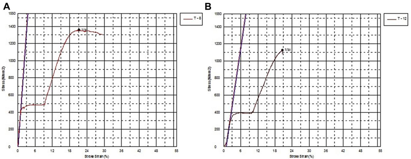
**Fig. 2.** Stress/strain curves in tensile test at T1. (A) Thermoelastic NiTi wire. (B) Pseudoelastic NiTi wire. The red line in the figures determines the slopes of the plots for continued loading before the thermoelastic region.
