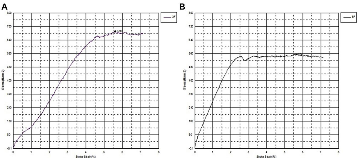
**Fig. 3.** Stress/strain curves in bending test at T0. (A) Thermoelastic NiTi wire. (B) Pseudoelastic NiTi wire. The red line in the figures determines the slopes of the plots for continued loading beyond the pseudoelastic region.
